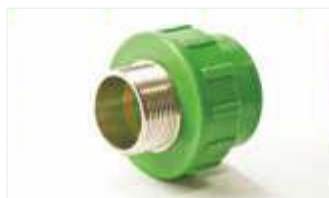
Male Threaded Adaptor 20mm*1/2" / 20mm*3/4" / 25mm*1/2" / 25mm*3/4" / 32mm*1/2" / 32mm*3/4" / 32mm*1" / 40mm*1.1/4" / 50mm*1.1/2" / 63mm*2", PN20
